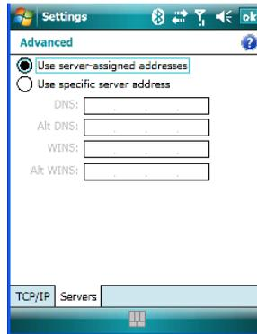
Servers requiring assigned IP addresses may also need a way to map computer names to IP addresses. The WORKABOUT PRO supports a variety of name resolution options: DNS, Alt DNS, WINS and Alt WINS.
